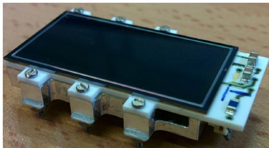
**Figure 3.** New SDD X-ray detectors for SIDDHARTA2 with a cell area of  $64\text{ mm}^2$ , total area of  $512\text{ mm}^2$ . The detectors will be cooled to about 170K and have a drift time of smaller than 500ns.
