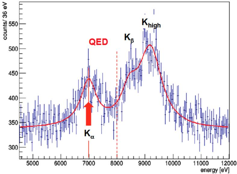
**Figure 4.** GEANT4 simulated kaonic deuterium X-ray spectrum (the pure electromagnetic  $2p-1s$  transition is indicated by an arrow) with a detector active area of  $246 \text{ cm}^2$  and assuming  $\epsilon_1 s = -800 \text{ eV}$  and  $\Gamma_1 s = 800 \text{ eV}$  [19]. With a  $K_{alpha}$  yield of 0.1 percent the signal-to-background ratio is 1:4.
