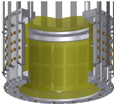
**Figure 2.** Design of the gas volume of SIDDHARTA 2 which provides the mandatory stability and the transmission for X-rays. The volume will be surrounded by arrays of X-ray detectors and shielding devices.
