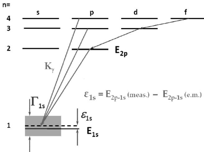
**Figure 1.** Transitions to the 1s ground state in kaonic hydrogen. Only the 1s state is measurably influenced by the strong antikaon-nucleon interaction. The calculated electromagnetic transition energy is about 6.5 keV which can be precisely measured with SDDs.
