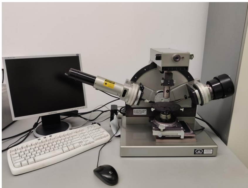
Slika 15. Elipsometar Gaertner Scientific Ellipsometer L116B-USB
