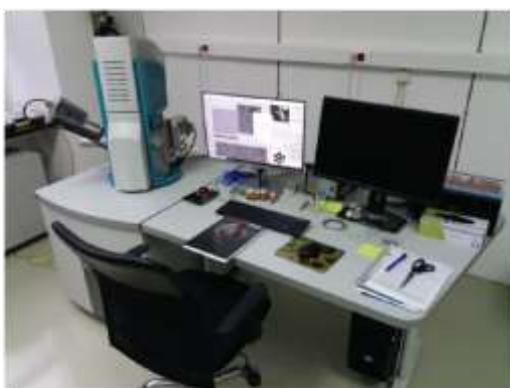
*Figure 22. Photograph of SEM at IFZg.*
