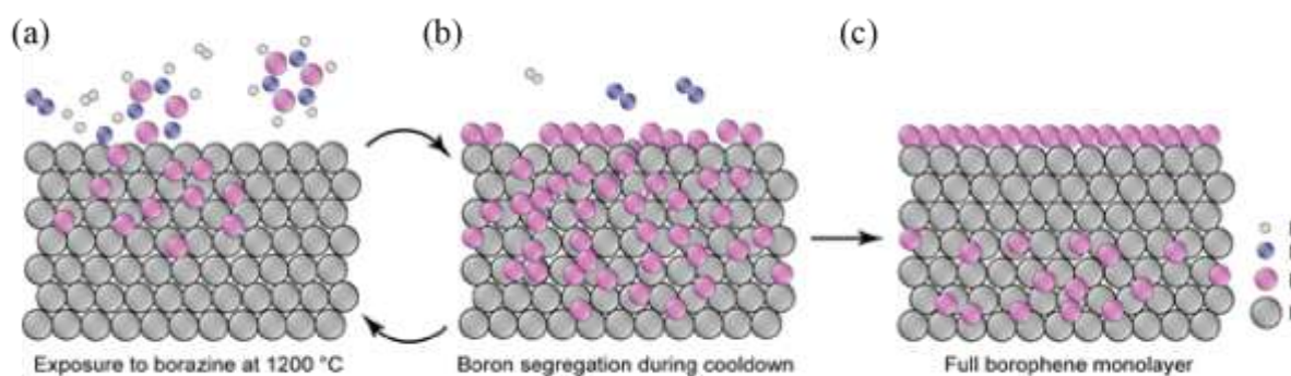
Figure 16. Schematic of segregation-enhanced epitaxy of Bo on Ir(111). (a) Borazine precursor is dosed repeatedly onto the hot Ir surface, resulting in boron dissolution into the bulk. (b) Sample cooldown follows each dosing step, during which B atoms segregate to the surface and self-assemble into a Bo mesh. (c) After finishing a set of dosing/cooling cycles, a full Bo monolayer is formed on the surface. [Adopted from Ref. 133 ].
