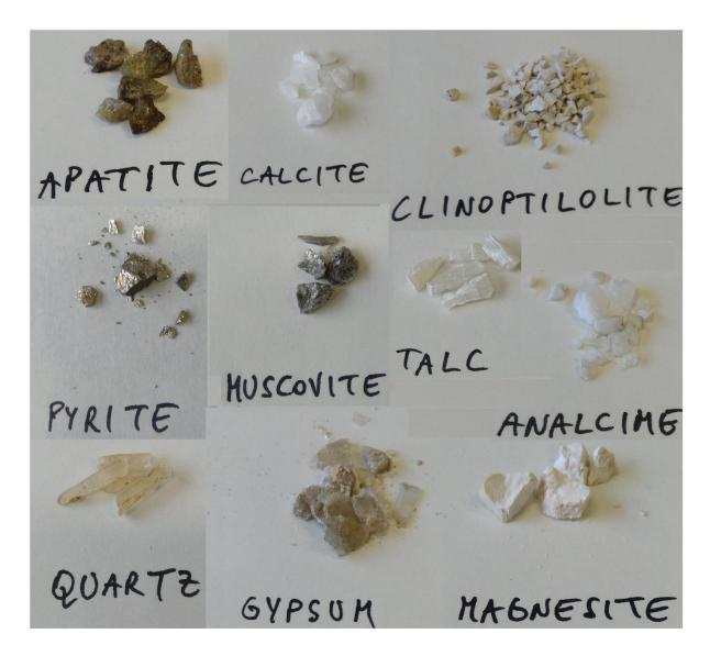
**Figure 42.** Mineral samples that were used in this study.
