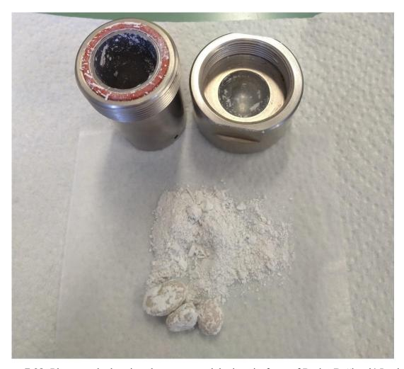
**Figure 7.38.** Photograph showing three stones picked up in front of Ruđer Bošković Institute by Prof. José G. Hernández. These stones were used as a milling media for milling Gly with TiO<sub>2</sub> for 18h at 20 Hz and ambient temperature. Gly oligomers up to Gly<sub>4</sub> were formed in this way.
