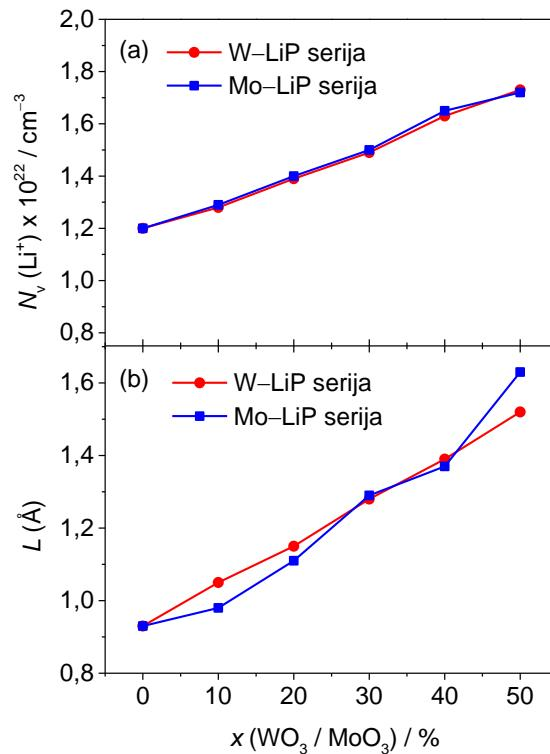
Slika 56. (a) Gustoća broja litijevih iona,  $N_v (\text{Li}^+)$ , i (b) Sidebottomova duljina,  $L$ , u ovisnosti o udjelu  $\text{WO}_3$  i  $\text{MoO}_3$  u serijama stakala  $x\text{WO}_3\text{-}40\text{Li}_2\text{O}\text{-(}60-x\text{)}\text{P}_2\text{O}_5$  i  $x\text{MoO}_3\text{-}40\text{Li}_2\text{O}\text{-(}60-x\text{)}\text{P}_2\text{O}_5$ ,  $x = 0\text{-}50\%$ .
