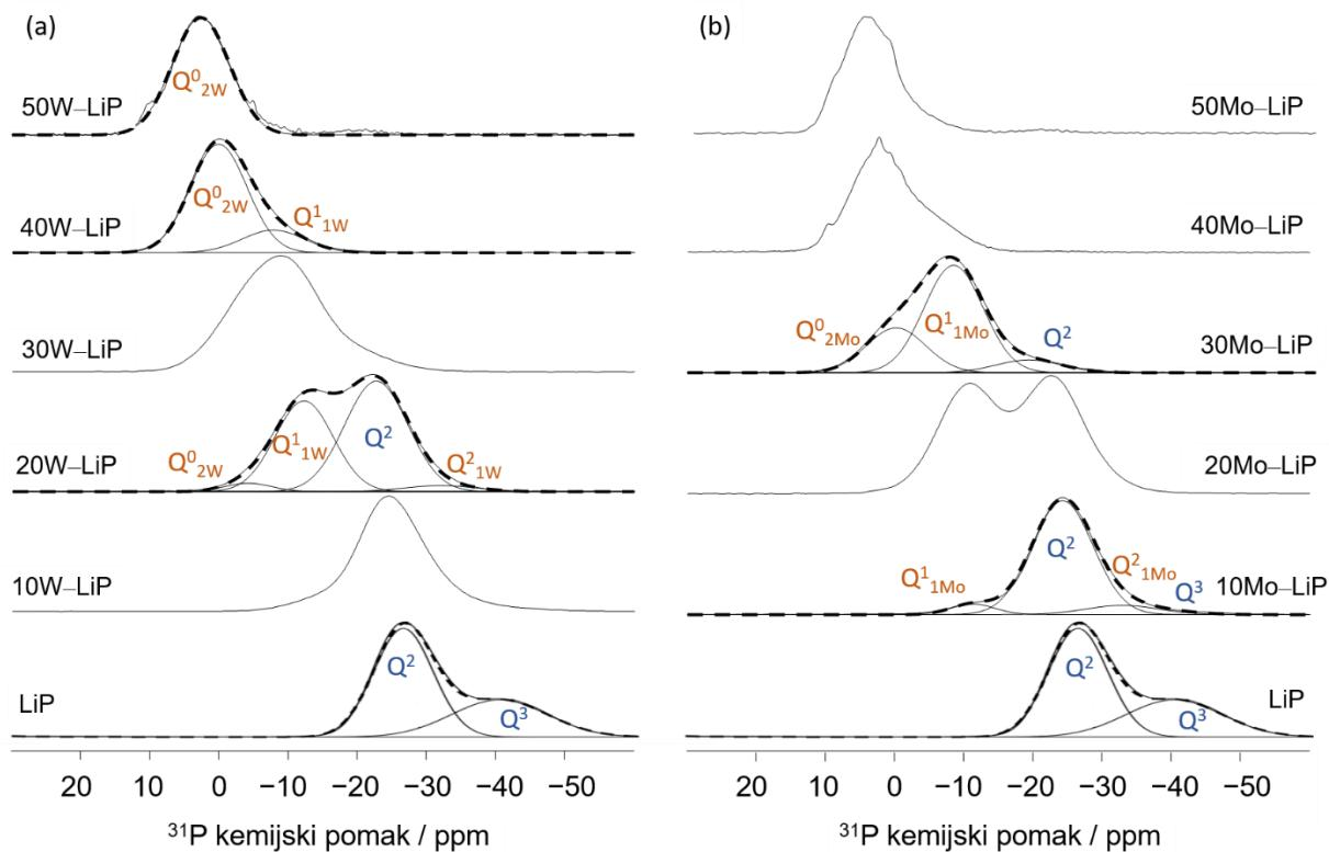
Slika 46.  $^{31}\text{P}$  MAS-NMR spektri serija stakala (a)  $x\text{WO}_3\text{-}40\text{Li}_2\text{O}\text{-}(60-x)\text{P}_2\text{O}_5$  i (b)  $x\text{MoO}_3\text{-}40\text{Li}_2\text{O}\text{-}(60-x)\text{P}_2\text{O}_5$ ,  $x=0\text{-}50\%$ .
