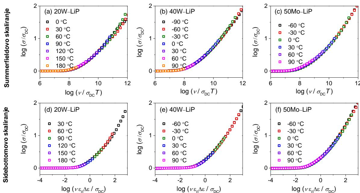
Slika 54. Spektri provodnosti 20W–LiP, 40W–LiP i 50Mo–LiP stakala iz serija  $x\text{WO}_3\text{--}40\text{Li}_2\text{O}\text{--}(60-x)\text{P}_2\text{O}_5$  i  $x\text{MoO}_3\text{--}40\text{Li}_2\text{O}\text{--}(60-x)\text{P}_2\text{O}_5$ ,  $x = 0\text{--}50\%$ , skalirani primjenom (a–c) Summerfieldovog i (d–f) Sidebottomovog postupka.
