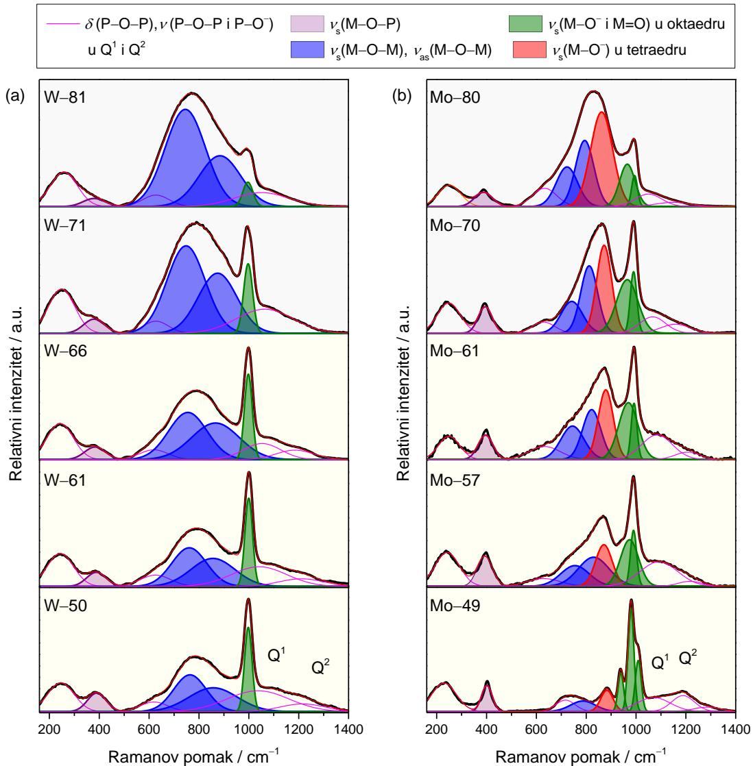
Slika 33. Ramanovi spektri serija stakala (a)  $x\text{WO}_3-(100-x)\text{P}_2\text{O}_5$  i (b)  $x\text{MoO}_3-(100-x)\text{P}_2\text{O}_5$ ,  $x = 49-81 \%$ .
