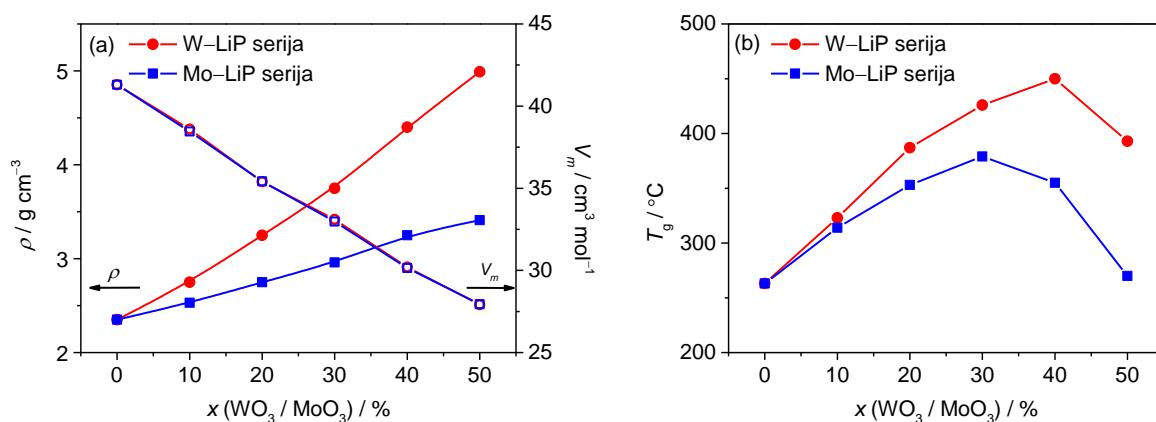
Slika 44. Ovisnost (a) gustoće,  $\rho$ , i molarnog volumena,  $V_m$ , te (b) temperature staklišta,  $T_g$ , o množinskom udjelu  $\text{WO}_3$  i  $\text{MoO}_3$  u serijama stakala  $x\text{WO}_3-40\text{Li}_2\text{O}-(60-x)\text{P}_2\text{O}_5$  i  $x\text{MoO}_3-40\text{Li}_2\text{O}-(60-x)\text{P}_2\text{O}_5$ ,  $x = 0-50 \%$ .
