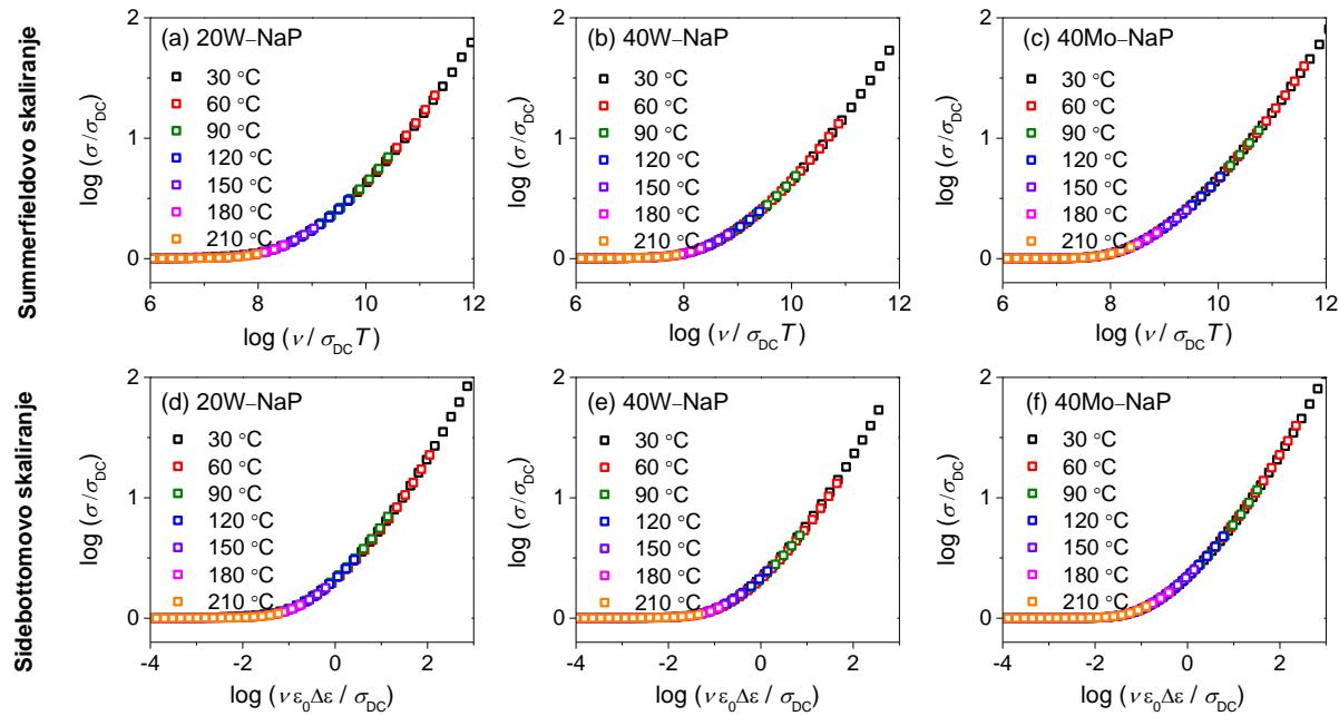
Slika 70. Spektri provodnosti 20W–NaP, 40W–NaP i 40Mo–NaP stakala iz serija  $x\text{WO}_3$ –40Na<sub>2</sub>O–(60– $x$ )P<sub>2</sub>O<sub>5</sub> i  $x\text{MoO}_3$ –40Na<sub>2</sub>O–(60– $x$ )P<sub>2</sub>O<sub>5</sub>,  $x = 0$ –50 %, skalirani primjenom (a–c) Summerfieldovog i (d–f) Sidebottomovog postupka.
