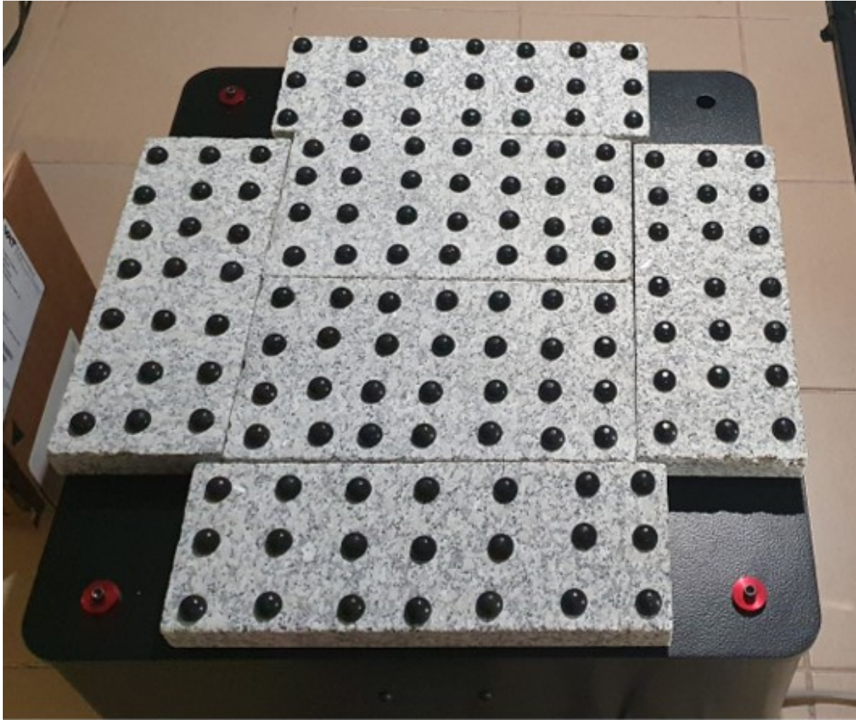
Figure 4.2: Installation of granite plates onto the anti-vibrational platform to reduce the overall load on the platform. Multiple dia-sorbothane hemisphere rubber bumpers were installed on both sides of the granite plates to ensure proper weight distribution across the entire platform.
