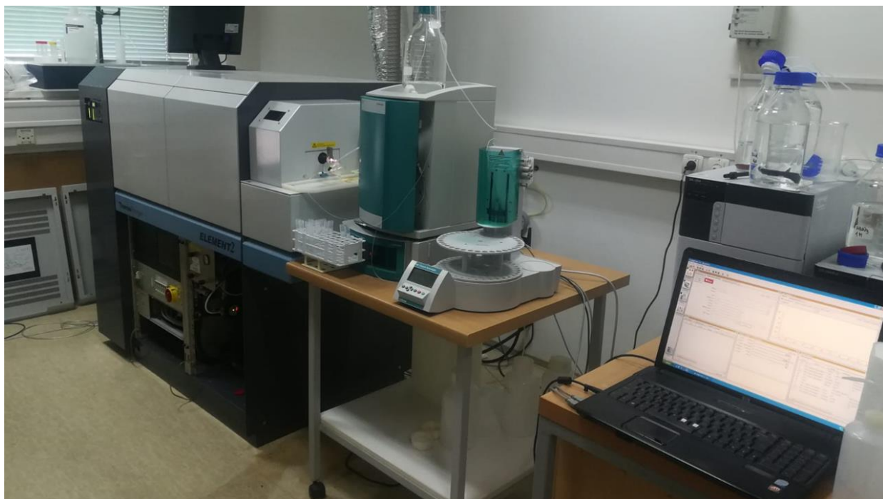
Figure 5. Example of connected IC to HR ICP-MS instrumentation in a single analytical system (“on-line” configuration). This instrumentation was used in determination of V redox species in the water samples of Krka River estuary (Research paper I.), at Ruđer Bošković Institute (Zagreb, Croatia).
