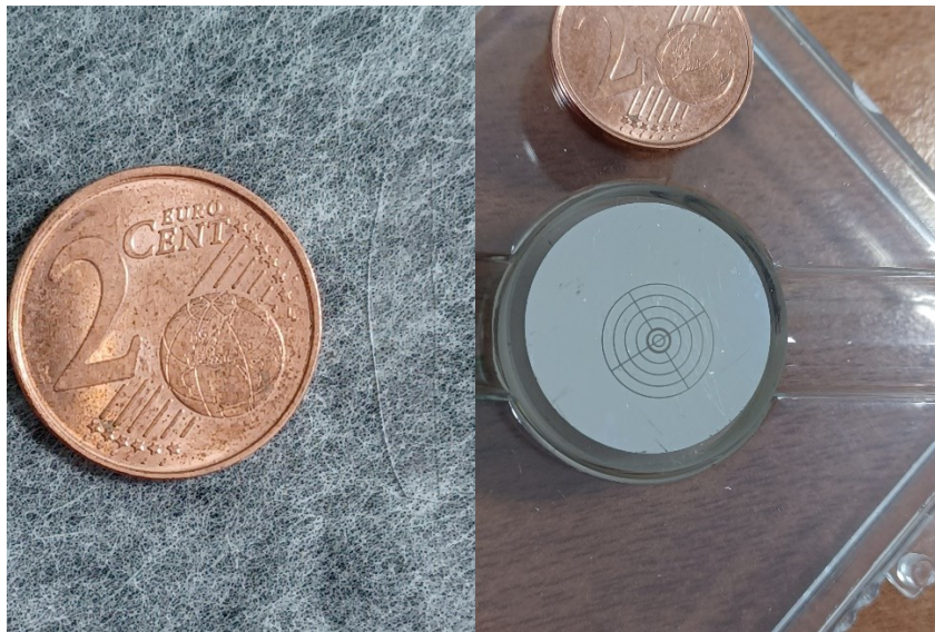
Figure 20. Left: part of a microscope cover glass; and right: silver mirror with a laser written pattern. The two-cent coin is used as an illustration of the size of the objects.
