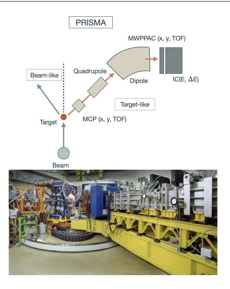
Figure 3.1: Schematic layout (top) and corresponding photo (bottom) of the PRISMA magnetic spectrometer when was coupled to CLARA  $\gamma$  array. The position of the detectors (MCP, MWPPAC and IC) in PRISMA and the physical quantities obtained with them, as well as the position of the magnets (quadrupole and dipole) are indicated in schematic layout.
