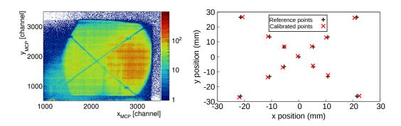
Figure 4.1: Matrix of the y vs. x position of MCP detector given in raw format, in channels (left) and calibration plot with reference and calibrated points (right).
