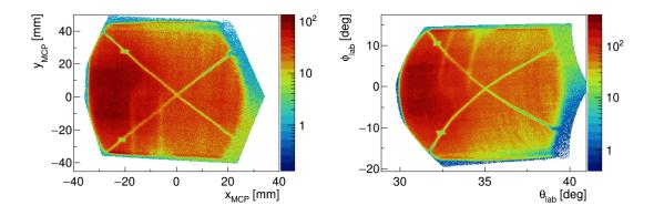
Figure 4.2: Matrices of the calibrated MCP detector in Cartesian (left) and angular (right) coordinates with coincidence with the focal plane detector MWPPAC.
