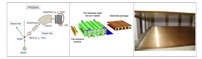
Figure 3.4: The position at PRISMA (left), schematic layout (center), and photo (right) of the ionizaton chamber. At the schematic layout, parts of detector are denoted: electrode package, the stainless-steel vacuum vessel and the entrance window.
