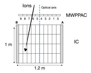
Figure 4.5: Shematic layout of the focal plane detectors of PRISMA. The side pads of the IC are in grey.
