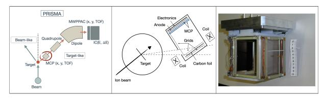
Figure 3.2: The position at PRISMA (left), schematic layout (center), and photo (right) of the MCP detector. At the schematic layout, parts of detector are denoted: carbon foil, two MCPs, anode, electronics and two external coils.
