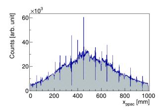
Figure 4.3: Calibrated spectrum of the position in the MWPPAC detector.
