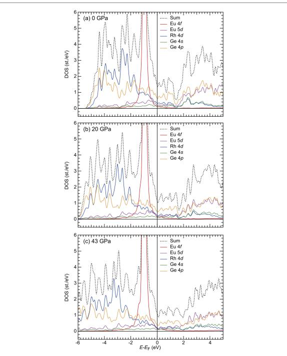
**Figure 3.** Total and partial density of states (DOS) calculated for EuRhGe<sub>3</sub> by DFT + U(U = 3.8 eV) at (a) 0 GPa, (b) 20 GPa, and (c) 43 GPa. In EuRhGe<sub>3</sub>, Ge atoms occupy two different crystallographic sites [16]. Here, the PDOS of all Ge atoms are plotted together.
