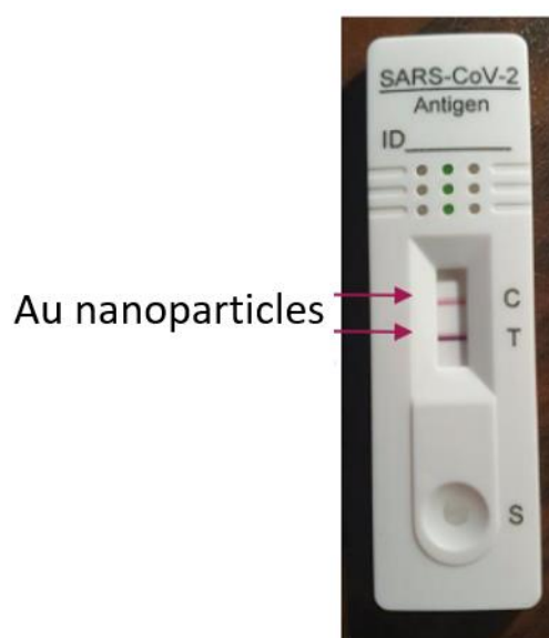
Figure 17. A lateral flow test with two visible red lines formed by accumulation of plasmonic Au nanoparticles. Picture courtesy of dr. Juraj Nikolić.
