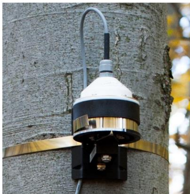
Slika 10. Digitalni denrometar (“Sap flow system EMS 81. Installation guide.,” 2018)
