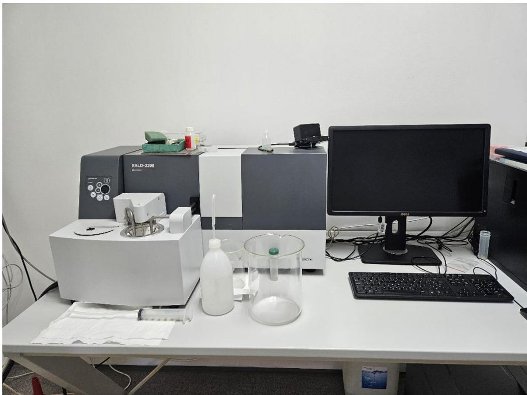
Figure 4.10 Shimadzu SALD-2300 laser diffraction particle size analyzer.
