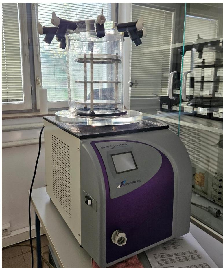
Figure 4.8 SP Scientific VirTis BenchTop Pro Freeze Dryer.
