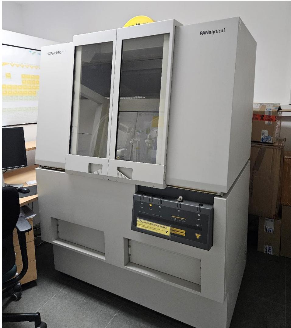
Figure 4.11 X-ray diffractometer PANalytical X'Pert Powder.
