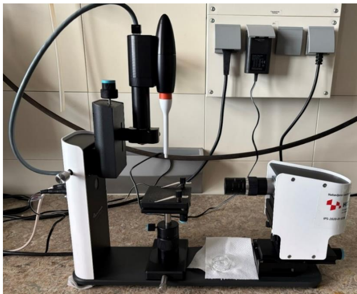
Slika 16. Tenziometar Attension Theta Lite ( Biolin Scientific ).
