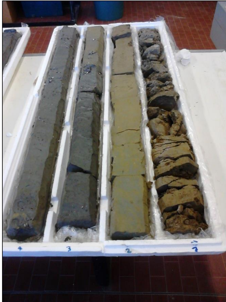
Figure 6.5. Deposits of continental and brackish environments in the first 4 m of the core MIR1.
