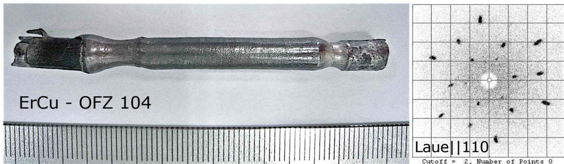
Figure 1.9: ErCu crystal prepared using optical floating zone technique with its Laue image in  $\langle 110 \rangle$  direction.
