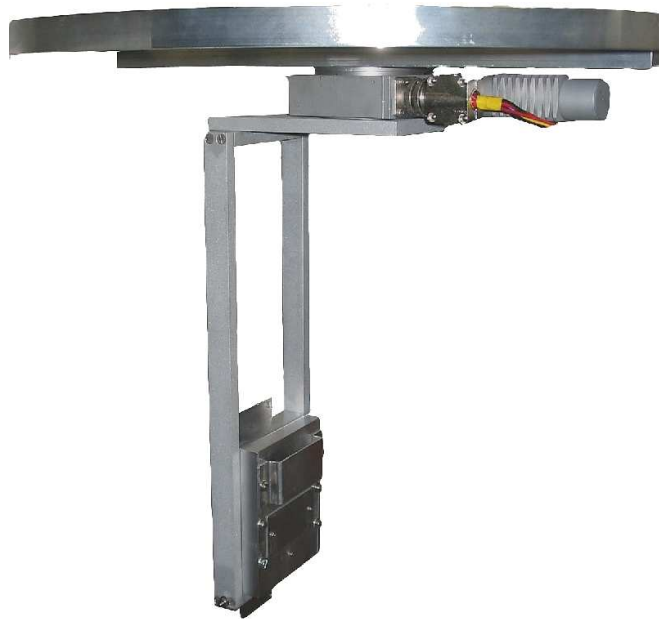
Figure 3.9: The detector housing and the supporting construction with the rotation motor.
