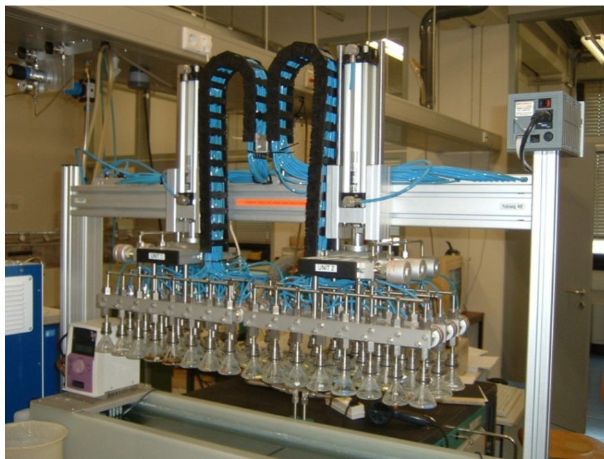
Figure 5.18 Set of 48 bottles prepared for water equilibration in water bath at constant temperature.
