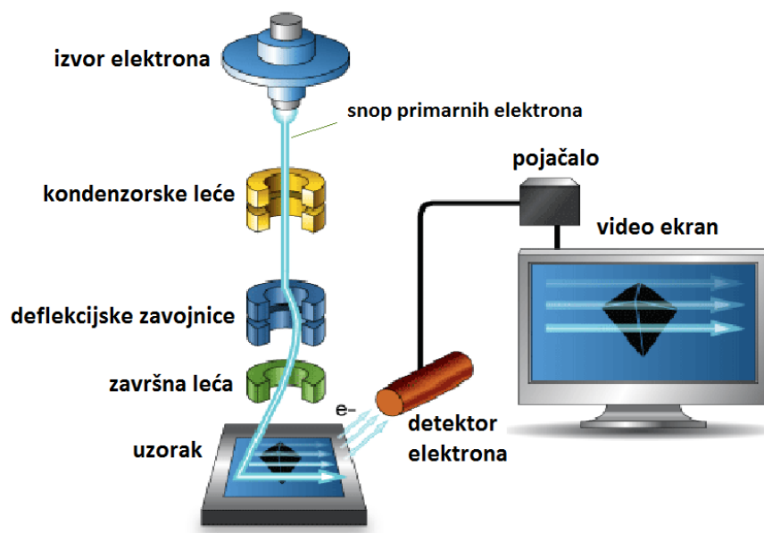
Slika 1. Prikaz sheme rada SEM instrumenta (preuzeto sa: MyScope (AMMRF), http://www.ammrf.org.au/myscope/sem/practice/principles/layout.php )
