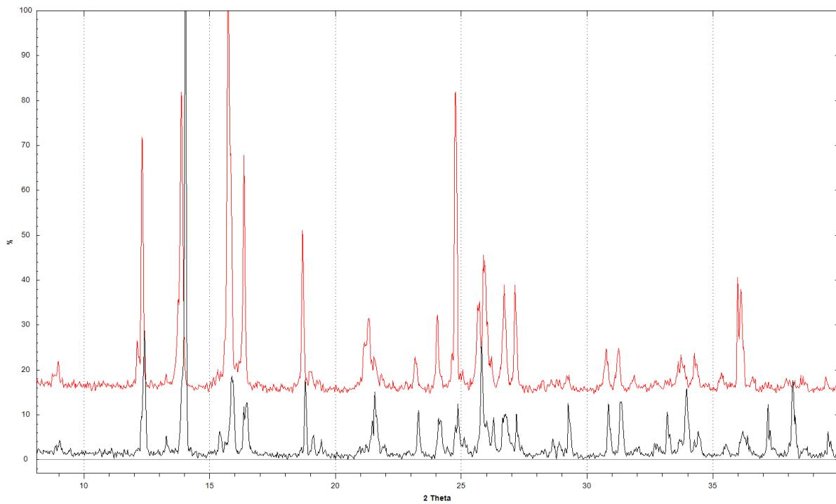
**Slika xxvi.** Difraktogram praha spoja  $[\text{CoC}_2\text{O}_4(\text{NH}_3)_4]\text{[Fe(C}_2\text{O}_4)_2(\text{OH}_2)_2 \cdot 2\text{H}_2\text{O}$  (crno) nastalog transformacijom iz kristala spoja  $[\text{Co}(\text{NH}_3)_6]\text{[Fe(C}_2\text{O}_4)_3]$ , u sintezi 3.3.2.; generirani difraktogram praha spoja  $[\text{CoC}_2\text{O}_4(\text{NH}_3)_4]\text{[Fe(C}_2\text{O}_4)_2(\text{OH}_2)_2 \cdot 2\text{H}_2\text{O}$  (crveno).
