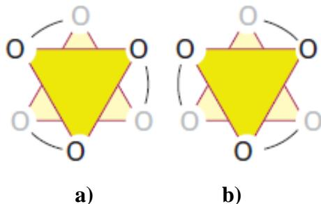
**Slika 6.** Apsolutna konfiguracija: a)  $\Delta\text{-}[\text{Fe}(\text{C}_2\text{O}_4)_3]^{3-}$  i b)  $\Lambda\text{-}[\text{Fe}(\text{C}_2\text{O}_4)_3]^{3-}$ .<sup>12</sup>
