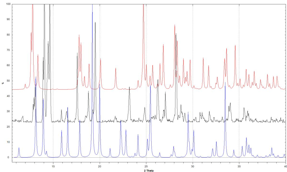
**Slika xx.** Generirani difraktogrami praha spojeva  $[\text{CoC}_2\text{O}_4(\text{NH}_3)_4]\text{[Fe(C}_2\text{O}_4)_2(\text{OH}_2)_2] \cdot \text{H}_2\text{O}$  (crno),  $\text{K}_3\text{[Fe(C}_2\text{O}_4)_3] \cdot 3\text{H}_2\text{O}$  (crveno) i  $\text{[CoC}_2\text{O}_4(\text{NH}_3)_4]\text{NO}_3 \cdot \text{H}_2\text{O}$  (plavo).
