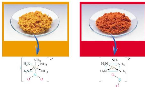
**Slika 11.** Vezni izomeri – žuti  $[\text{Co}(\text{NH}_3)_5(\text{NO}_2)]\text{Cl}_2$  i crveni  $[\text{Co}(\text{NH}_3)_5(\text{ONO})]\text{Cl}_2$ .<sup>4</sup>
