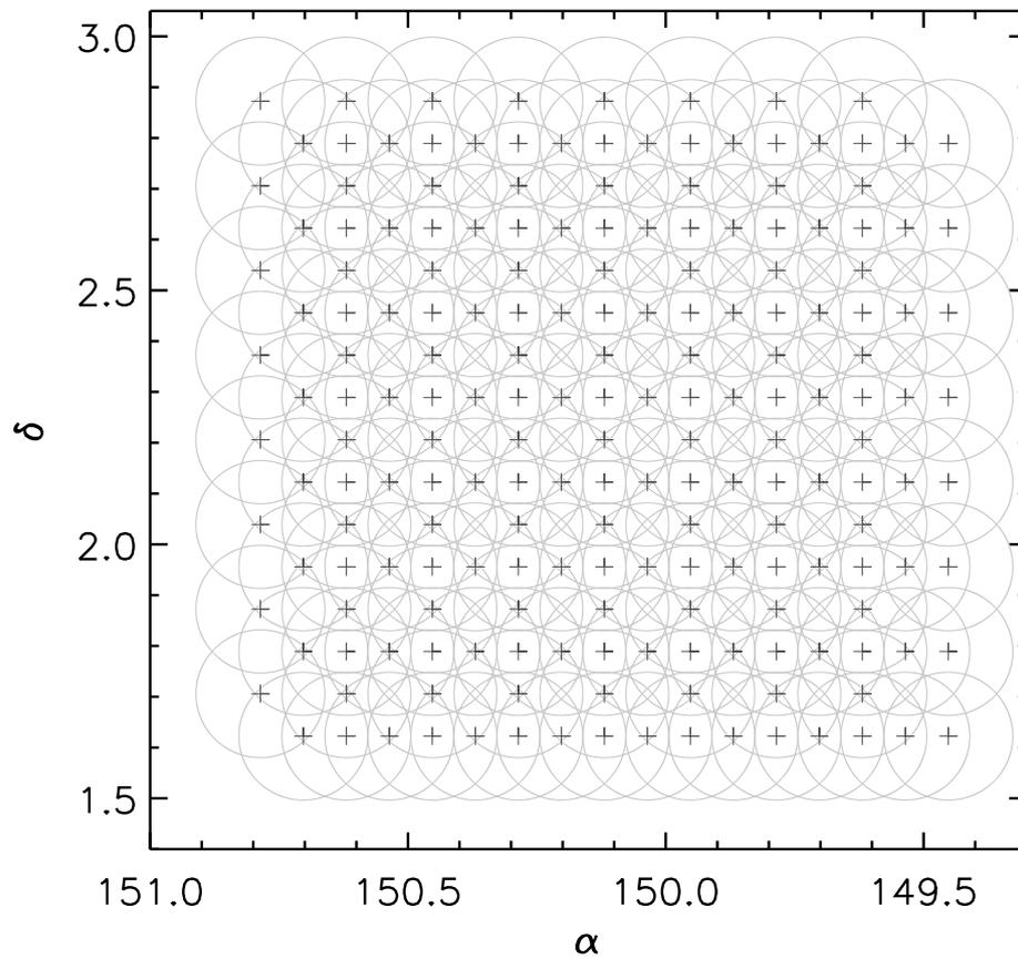
Figure 3.2: Pointing pattern used for the 3 GHz VLA-COSMOS Large Project. The centers of the 192 pointings are indicated by the plus signs. Circles indicate the primary beam of each pointing, represented here by the HPBW at 3 GHz ( $15'$ ; the primary beam HPBW is a function of frequency and varies by a factor 2 between the lower and upper edge of the S band).
