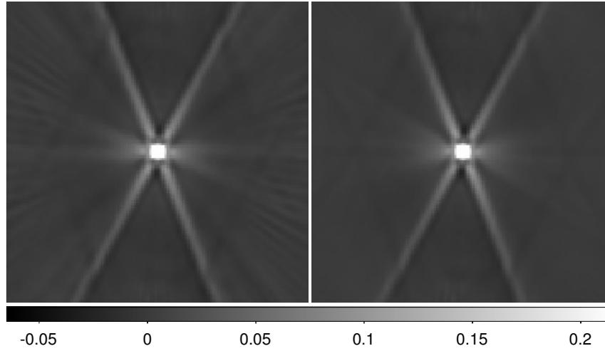
Figure 3.5: *Left panel*: final (A- plus C-array configuration combined) dirty beam of one pointing, after tapering. This beam was used in the cleaning of that pointing (see text for details). *Right panel*: mean stack of all 192 dirty beams. The contribution of radial sidelobes is 10% at maximum.
