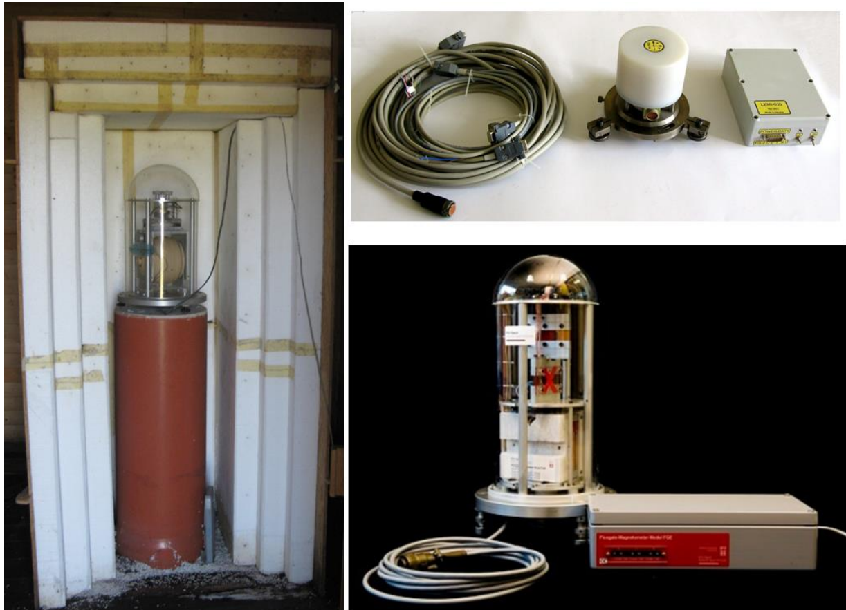
Figure 2.1 Left: Variometer based on a scalar magnetometer; a suspended dIdD magnetometer (manufacturer: GEM Systems, Canada), the main variometer at LON. Top-right: LEMI-035, three-component fluxgate magnetometer, the supplement variometer at LON (manufacturer: Lviv Centre of Institute for Space Research). Bottom-right: FGE, a very popular type of the suspended three-component fluxgate magnetometer (manufacturer: Danish Meteorological Institute, DMI). This type of instrument is used in many observatories worldwide.
