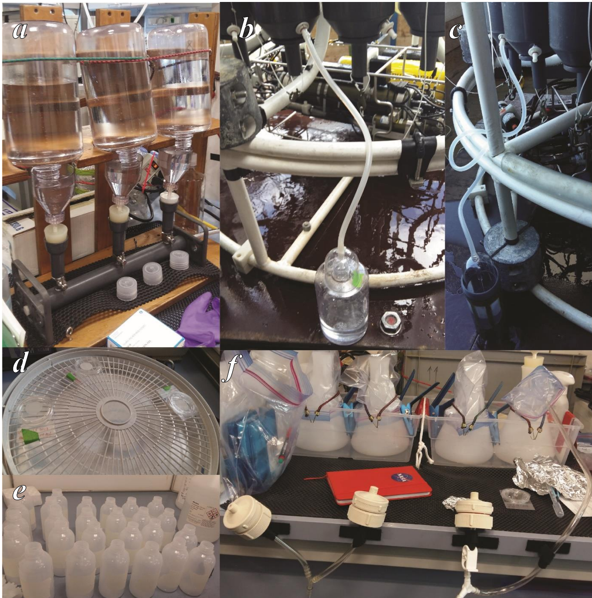
Fig. 10. Sampling and filtration methods: a) sample filtration for HPLC; b) subsampling from CTD probe (pigment and phytoplankton analysis); c) filtration from Niskin bottles; d) filter excitation; e) bottle preparation for phytoplankton; f) sample filtration for SEM.
