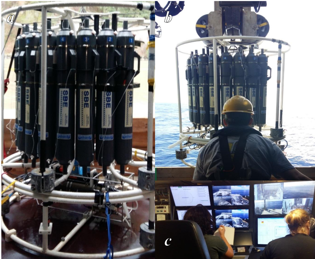
Fig. 9. a) Niskin bottles with CTD probes arranged in a rosette; b) rosette recovery from the ocean, c) CTD control room.
