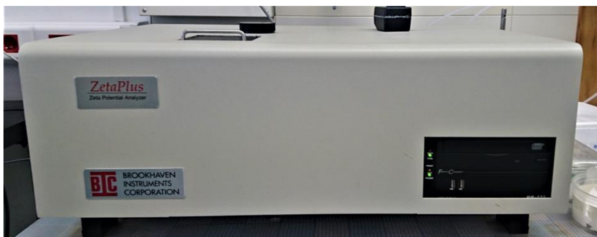
Slika 6. Zeta Plus, Particle Size Analyzer, Brookhaven Instrument Corporation
