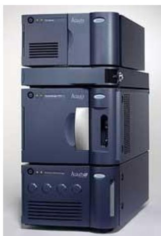
**Slika 5.** Instrument UHPLC
