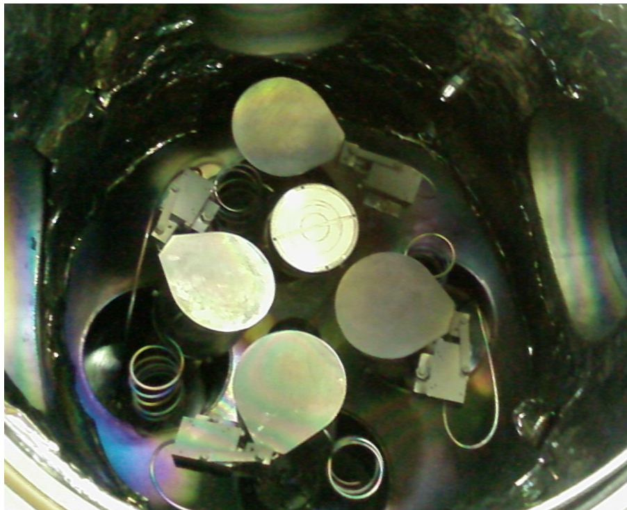
Figure 9. Magnetron sputtering chamber. Four magnetrons are shown, one without the lid has a gold target used mostly for the contact deposition. By moving the lids, we can control which material is deposited.
