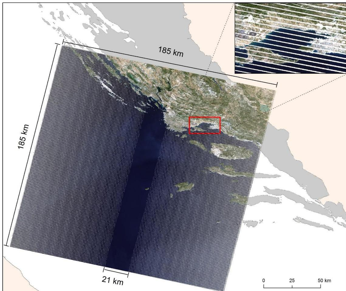
Sl. 7. Scena ETM+ senzora nakon kvara *scan line corrector* instrumenta
