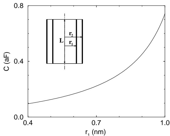
Fig. 3. Capacitance of a capacitor as a function of an internal radius  $r_1$ , for  $L = 2.6$  nm, and an external radius  $r_2 = 1.2$  nm. Inset: the geometry of a nanometer-scale cylindrical capacitor.
