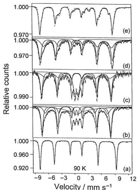
Figure 8.  $^{57}\text{Fe}$  Mössbauer spectra at 90 K of (a)  $\alpha\text{-Fe}_2\text{O}_3$ , (b) rust formed in 0.005 M  $\text{Na}_2\text{CO}_3$  at rt in one month, (c) rust formed in 0.005 M  $\text{Na}_2\text{CO}_3$  at rt in one week, (d) rust formed in doubly distilled water at 90 °C in three weeks, and (e)  $\text{Fe}_3\text{O}_4$ .  $\alpha\text{-Fe}_2\text{O}_3$  and  $\text{Fe}_3\text{O}_4$  are used as reference materials
