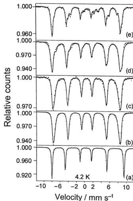
Figure 9.  $^{57}\text{Fe}$  Mössbauer spectra at 4.2 K of (a)  $\alpha\text{-Fe}_2\text{O}_3$ , (b) rust formed in 0.005 M  $\text{Na}_2\text{CO}_3$  at rt in one month, (c) rust formed in 0.005 M  $\text{Na}_2\text{CO}_3$  at rt in one week, (d) rust formed in doubly distilled water at 90 °C in three weeks and (e)  $\text{Fe}_3\text{O}_4$ .  $\alpha\text{-Fe}_2\text{O}_3$  and  $\text{Fe}_3\text{O}_4$  used as reference materials.
