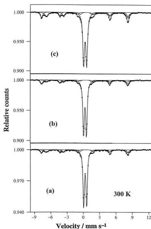
Figure 1. <sup>57</sup>Fe Mössbauer spectra at 300 K of rust formed after (a) one week, (b) three weeks and (c) six months of corrosion in doubly distilled water.
