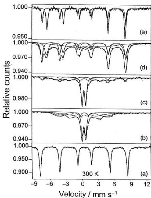
Figure 7.  $^{57}\text{Fe}$  Mössbauer spectra at 300 K of (a)  $\alpha\text{-Fe}_2\text{O}_3$ , (b) rust formed in 0.005 M  $\text{Na}_2\text{CO}_3$  at rt in one month, (c) rust formed in 0.005 M  $\text{Na}_2\text{CO}_3$  at rt in one week, (d) rust formed in doubly distilled water at 90 °C in 3 weeks, and (e)  $\text{Fe}_3\text{O}_4$ .  $\alpha\text{-Fe}_2\text{O}_3$  and  $\text{Fe}_3\text{O}_4$  used as reference materials.
