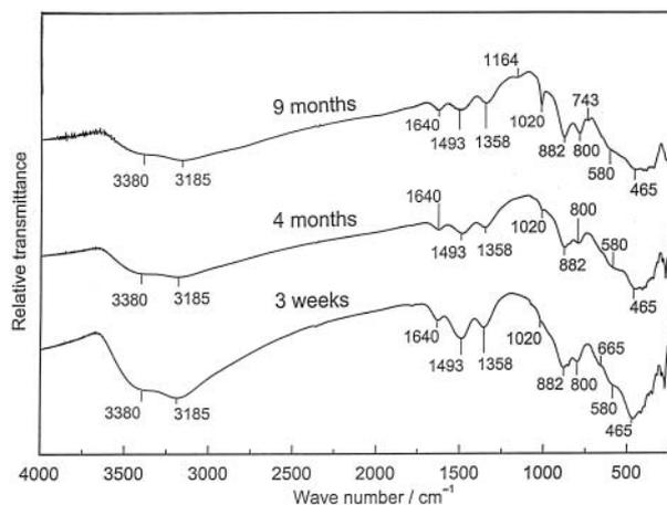
Figure 6. FT-IR spectra of rust formed after three weeks, four months and nine months of corrosion in natural water.
