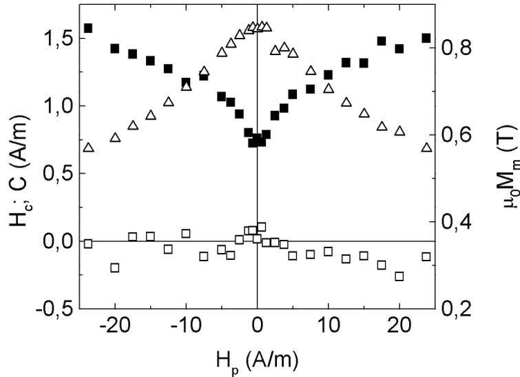
Fig. 7. Variations of the coercive field  $H_c$  (■), maximum magnetization  $M_m$  ( $\Delta$ ) and the position of the centre of the  $M-H$  loop  $C$  ( $\square$ ), for the nanocrystalline  $\text{Fe}_{73.5}\text{Cu}_1\text{Nb}_3\text{Si}_{15.5}\text{B}_7$  sample, with the static surface field  $H_p$ . The triangular magnetizing field with the amplitude  $H_0 = 10$  A/m and the frequency  $f = 5.5$  Hz was used.
