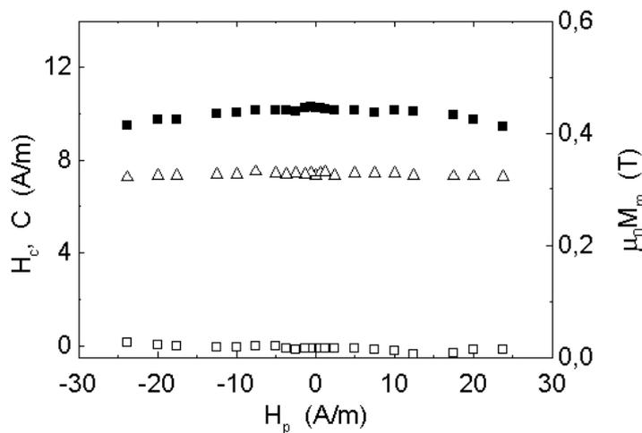
Fig. 4. Variation of the coercive field  $H_c$  (■), maximum magnetization  $\mu_0 M_m$  ( $\Delta$ ) and the position of the centre of the  $M - H$  loop  $C$  (□) with the magnitude of static surface field  $H_p$  for the  $\text{Fe}_{73.5}\text{Cu}_1\text{Nb}_3\text{Si}_{15.5}\text{B}_7$  ribbon in the amorphous state. A triangular drive field  $H$  with the frequency  $f = 5.5$  Hz and the amplitude  $H_0 = 25$  A/m was used.
