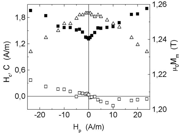
Fig. 6. Variations of the coercive field  $H_c$  (■), maximum magnetization  $M_m$  ( $\Delta$ ) and the position of the centre of the  $M-H$  loop  $C$  ( $\square$ ), for the nanocrystalline Fe<sub>73.5</sub>Cu<sub>1</sub>Nb<sub>3</sub>Si<sub>15.5</sub>B<sub>7</sub> sample, with the static surface field  $H_p$ . The triangular magnetizing field with the amplitude  $H_0 = 100$  A/m and the frequency  $f = 5.5$  Hz was used.
