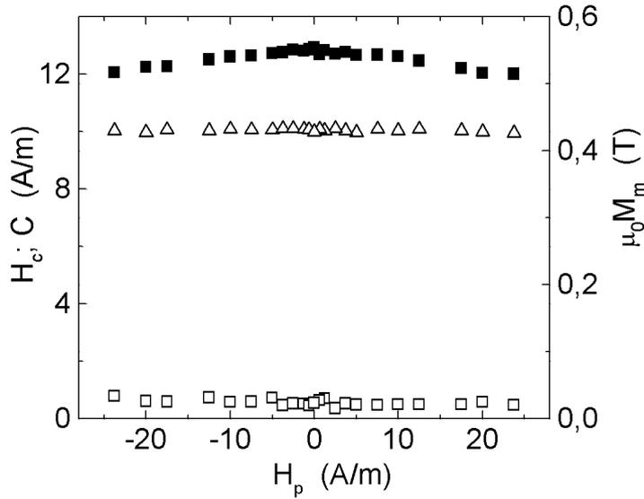
Fig. 3. Variation of the coercive field  $H_c$  (■), maximum magnetization  $\mu_0 M_m$  ( $\Delta$ ) and the position of the centre of the  $M - H$  loop  $C$  (□) with the magnitude of static surface field  $H_p$  for the  $\text{Fe}_{73.5}\text{Cu}_1\text{Nb}_3\text{Si}_{15.5}\text{B}_7$  ribbon in the amorphous state. A triangular drive field  $H$  with the frequency  $f = 5.5$  Hz and the amplitude  $H_0 = 100$  A/m was used.
