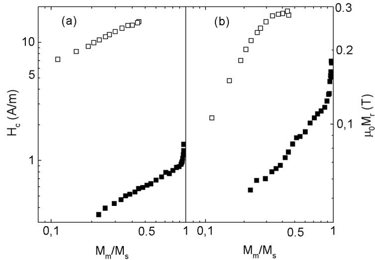
Fig. 2. Variation of the coercive field  $H_c$  (a) and remanent magnetization  $M_r$  (b) with the normalized magnetization  $M_m/M_s$  before annealing (open symbols) and after annealing at temperature  $T_a = 540^\circ \text{C}$  (solid symbols) for the  $\text{Fe}_{73.5}\text{Cu}_1\text{Nb}_3\text{Si}_{15.5}\text{B}_7$  ribbon. A triangular drive field  $H$  with the frequency  $f = 5.5$  Hz and different amplitudes  $H_0 \leq 350$  A/m was used.
