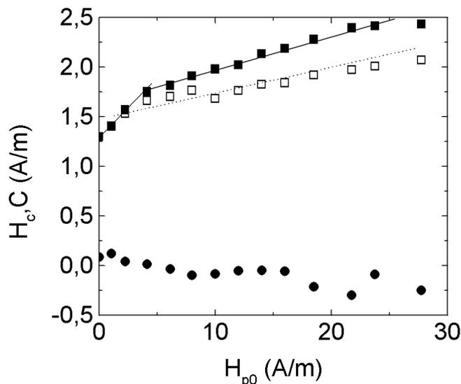
Fig. 8. Variation of the coercive field  $H_c$  with the amplitude of the dynamic surface field  $H_{p0}$ , for the suitable phase ( $\square$ ) and unsuitable phase ( $\blacksquare$ ) of  $H_p$  (see text). ( $\bullet$ ) represent the corresponding variation of the position of the centre of the  $M-H$  loop  $C$  for the suitable phase. The triangular magnetizing field with the amplitude  $H_0 = 100$  A/m and the frequency  $f = 5.5$  Hz was used.
