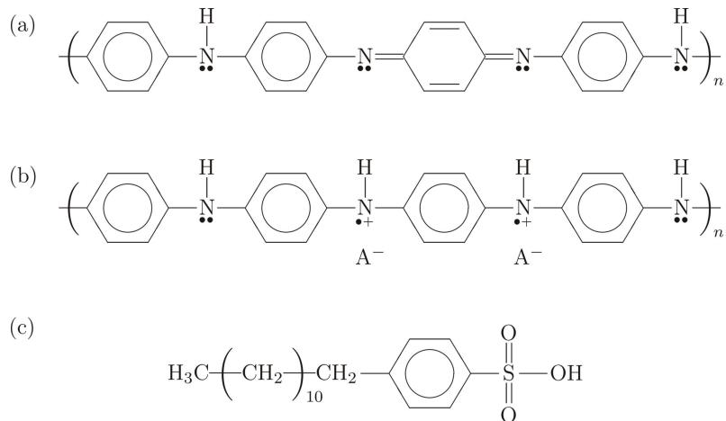
**Figure 1.** (a) One mer of PANI-EB. (b) One mer of fully protonated  $(\text{PANI-H})^+ \text{A}^-$ . (c) DBSA molecule.
