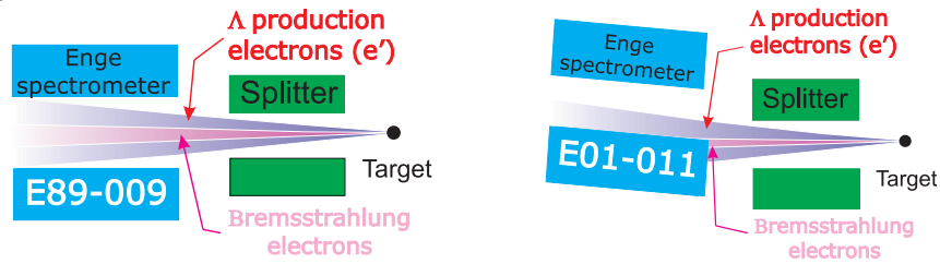
Fig. 4. ENGE configuration as used in E89-009: ENGE set in the Splitter plane, and for E01-001: ENGE had vertical offset and tilt with respect to the Splitter plane.
