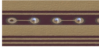
Figure 4.18: A detail of the prototype sample for laser soldering test: three solder balls of 250\ \mu\text{m} diameter placed on top of the chip and FPC prior to laser soldering are visible
