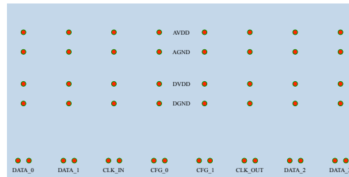
Figure 4.16: Sketch of principle of the connection pads array over the Pixel Chip top surface.
