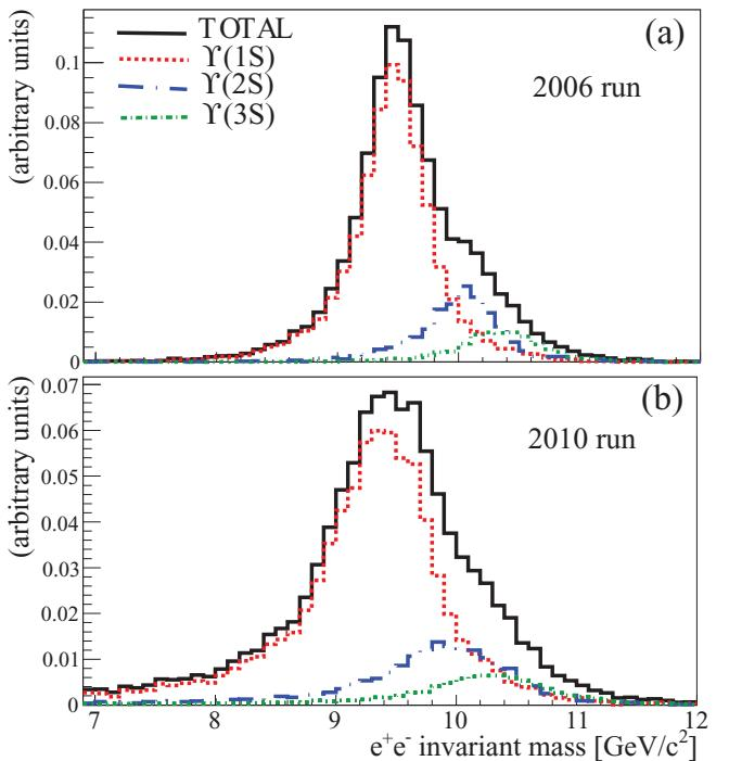
FIG. 4. (Color online) Invariant mass distribution of simulated  $\Upsilon(1S + 2S + 3S)$  using the PHENIX detector simulation and relative  $\Upsilon$  yields from CDF experiment [47] in the 2006 run (a) and the 2010 run (b) detector configurations.
