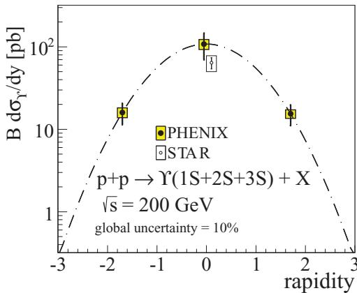
FIG. 10. (Color online) Rapidity dependence of  $\Upsilon(1S + 2S + 3S)$  yield measured by PHENIX, forward rapidity result from [53], and STAR midrapidity from [54]. The dashed line is a Gaussian function fitted to the points. The points at zero rapidity are shifted for clarity.
