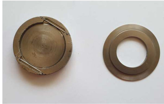
Figure 3.12. Metal holder for in-situ XRD measurements
