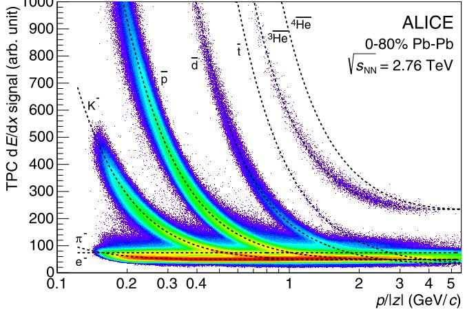
**Fig. 1.** TPC  $dE/dx$  spectrum for negative particles in a sample of three different trigger types (minimum bias, semi-central and central). The dashed lines are parametrisations of the Bethe–Bloch-formula [38–40] for the different particle species.
