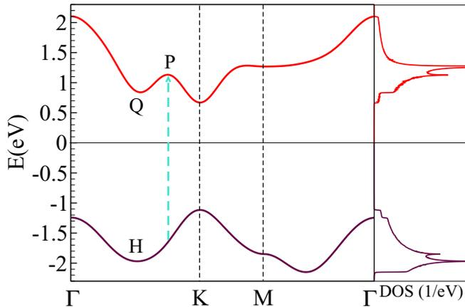
FIG. 4. The valence band (violet) and conduction band (red) and their density of states (right panel). Notice the saddle points at  $P$ ,  $H$  and  $M$  which give singular contribution to the density of states. The points  $Q$  and  $H$  are approximately at  $(2\pi/3a, 0)$  as noted in Ref. [32].
