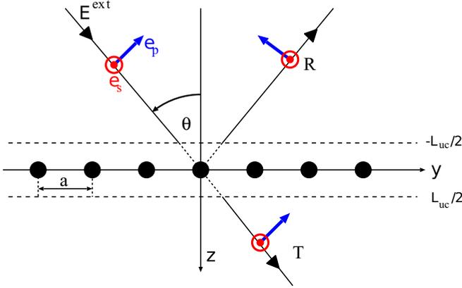
FIG. 1. Schematic description of the geometry of the system. The q2D crystal lies in the  $x$ - $y$  plane,  $a$  represents lattice constant in the  $x$ - $y$  plane and  $L_{uc}$  is the lattice constant in the  $z$  direction.  $\theta$  is incident angle of  $s$ (TE) and  $p$ (TM) polarized electromagnetic field.
