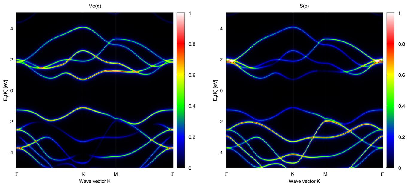
FIG. 2. The intensities of contributions of the Mo(*d*) orbital (left panel) and S(*p*) orbital (right panel) to MoS<sub>2</sub> band structure.
