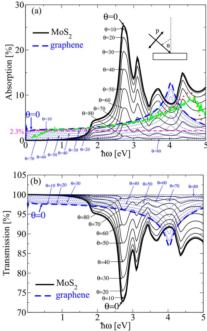
FIG. 6. Angle-resolved optical absorbance (a) and transmittance (b) in MoS<sub>2</sub> monolayer (black lines) and in graphene monolayer (blue dashed lines). The incident angle increases as  $\theta_n = n\Delta\theta$ ;  $n = 0, 1, \dots, 8$ , where  $\Delta\theta = 10^\circ$ , as denoted in the graphs. Normal incidence ( $\theta = 0$ ) absorbance in graphene taken from Ref. [18] (red dotted line) and Ref. [4] (green dashed-dotted line).
