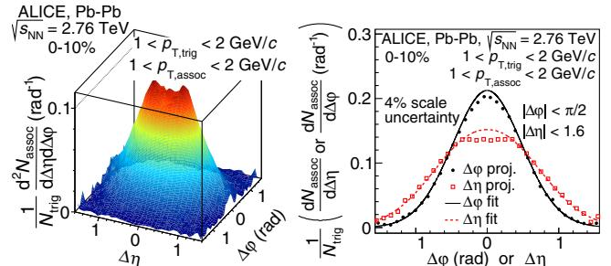
FIG. 1. Left panel: associated yield per trigger particle as a function of  $\Delta\varphi$  and  $\Delta\eta$ . The background obtained from the fit function has been subtracted in order to emphasize the near-side peak. Right panel: projections to the  $\Delta\varphi$  and  $\Delta\eta$  axes overlaid with the peak part of the fit function.
