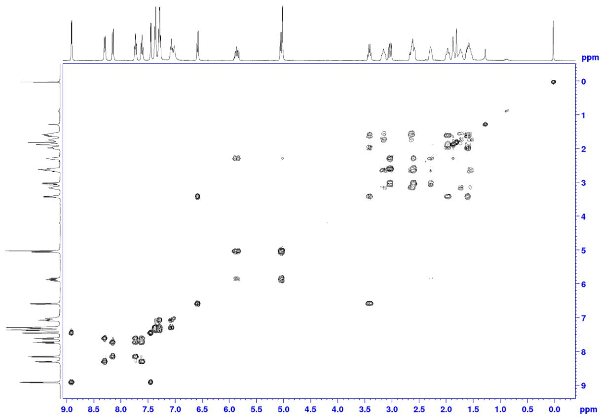
Slika D21. COSY spektar spoja **6** snimljen u  $\text{CDCl}_3$
