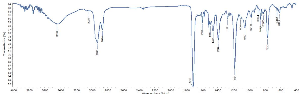
Slika D9. IR spektar spoja **3**
