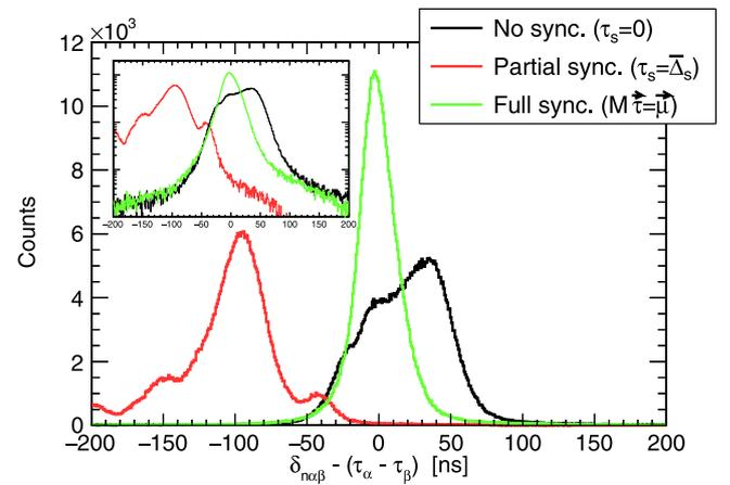
Fig. 7. Overall distribution of time differences between coincidental pulses from the measurement of the  ${}^6\text{Li}(n, t)$  reaction, registered by any pair of silicon strips. The partial synchronization based solely on Eq. (6) exacerbates the time offsets between the strips. The inset shows the plots in the logarithmic scale, facilitating the selection of  $\pm 100$  ns as a window width for the identification of coincidental pulse.
