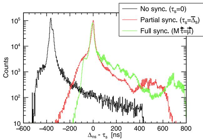
Fig. 3. Overall distribution of differences between the  $\gamma$ -flash instants as registered by a particular silicon strip and as registered by an external timing device (WCM). The synchronization procedure aims at identifying the set of offsets  $\tau_s$  such that the condition from Eq. (6) is satisfied, i.e. that the mean of the corrected spectra is as close to zero as possible. The full synchronization procedure takes into account further requirements from Eqs. (10) and (13).
