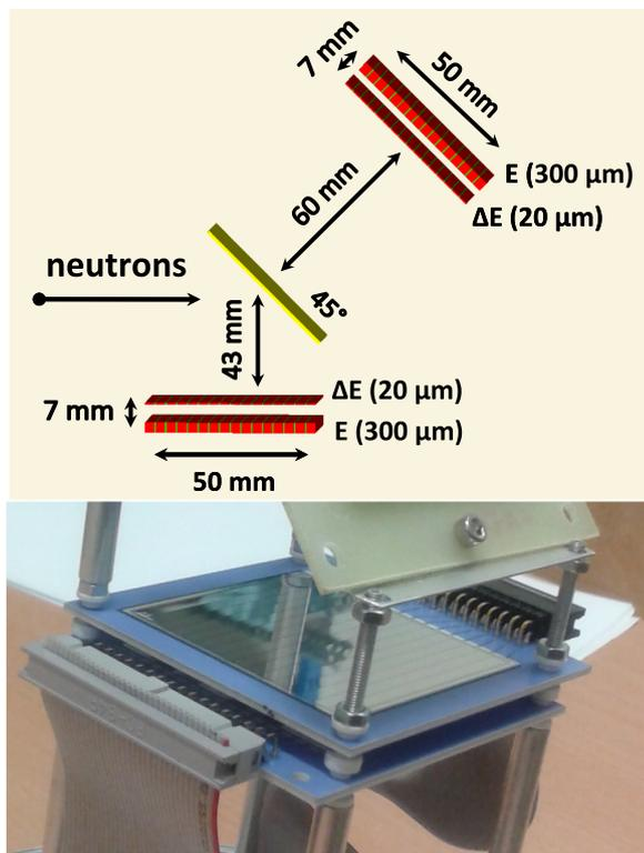
Fig. 1. Top: detector configuration from the joint measurement of the  $^{12}\text{C}(n,p)$  and  $^{12}\text{C}(n,d)$  reactions, comprising two identical silicon telescopes (all widths are exaggerated). At the center is the bearing structure for the LiF calibration sample (we use these calibration data in this work). Bottom: SITE close-up. The striped structure of  $\Delta E$ -layer (shown here) is clearly visible.
