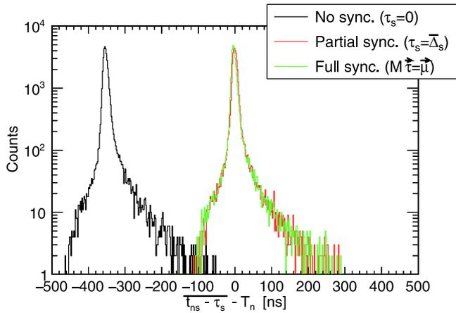
Fig. 5. Overall distribution of averaged  $\gamma$ -flash instants from Eq. (11), as registered by separate silicon strips. Already the partially synchronized spectrum – accounting only for the set of conditions from Eq. (6) – satisfies to a high degree the expectation from Eq. (12). Full synchronization considers this as an explicit requirement, alongside Eqs. (6) and (10).
