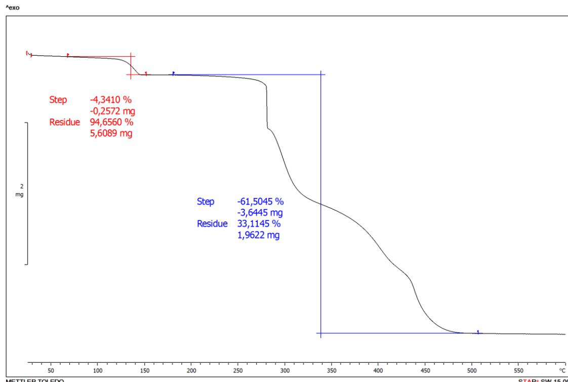
**Slika D8.** Termogravim spoja  $[\text{MoO}_2(\text{4OHSal-4HBOH})(\text{H}_2\text{O})]$
