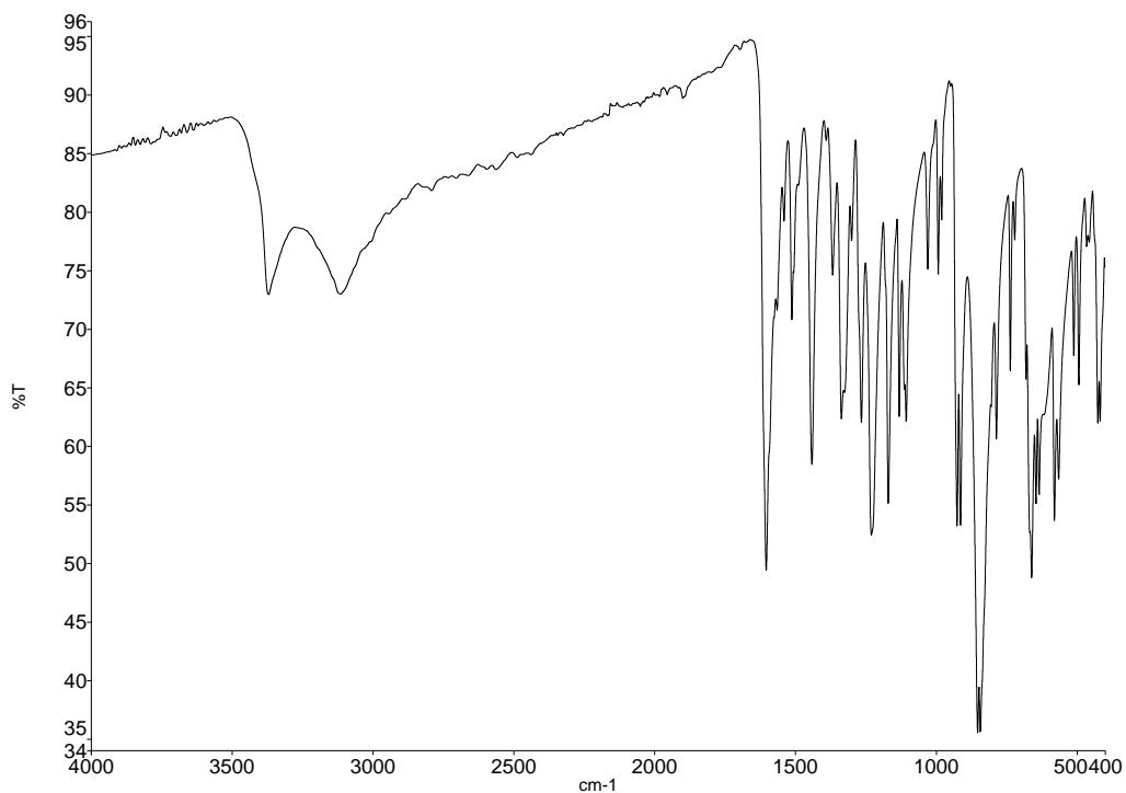
**Slika D19.** Infracrveni spektar polimernog spoja  $[\text{MoO}_2(\text{4OHSal-4HBOH})]_n$
