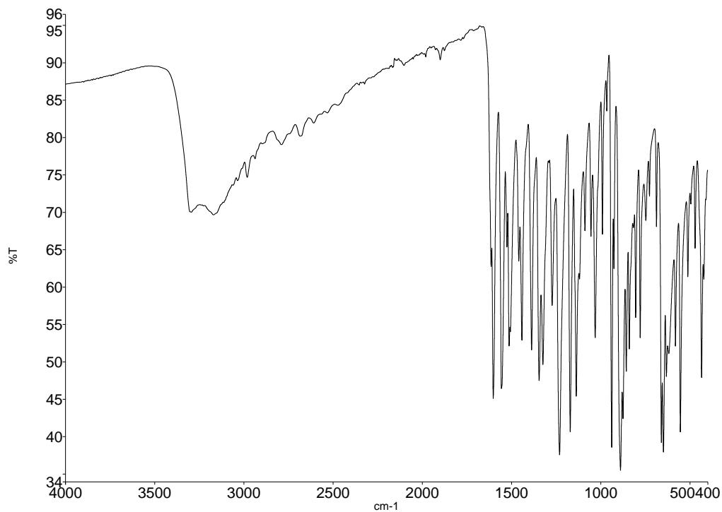
**Slika D30.** Infracrveni spektar kompleksa  $[\text{MoO}_2(\text{4OHSal-4HBOH})(\text{EtOH})]$  dobiven transformacijom polimera  $[\text{MoO}_2(\text{4OHSal-4HBOH})]_n$  u parama etanola
