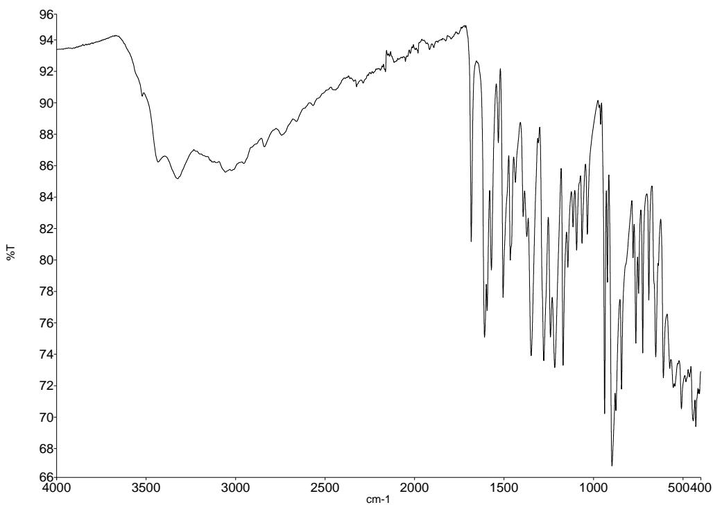
**Slika D20.** Infracrveni spektar kompleksa  $[\text{MoO}_2(\text{3OHSal-4HBOH})(\text{H}_2\text{O})] \cdot (\text{CH}_3)_2\text{CO}$
