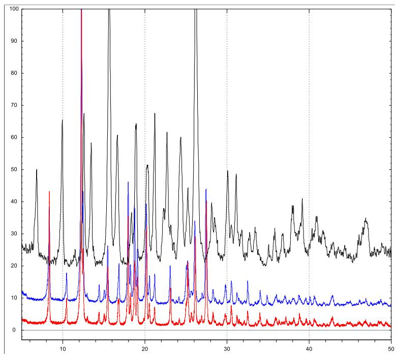
**Slika 23.** Usporedba difraktograma prahova:  $[\text{MoO}_2(\text{3OHSal-4HBOH})(\text{EtOH})] \cdot \text{EtOH}$  (crno),  $[\text{MoO}_2(\text{3OHSal-4HBOH})(\text{EtOH})]$  (crveno), transformacija polimera u parama etanola (plavo)
