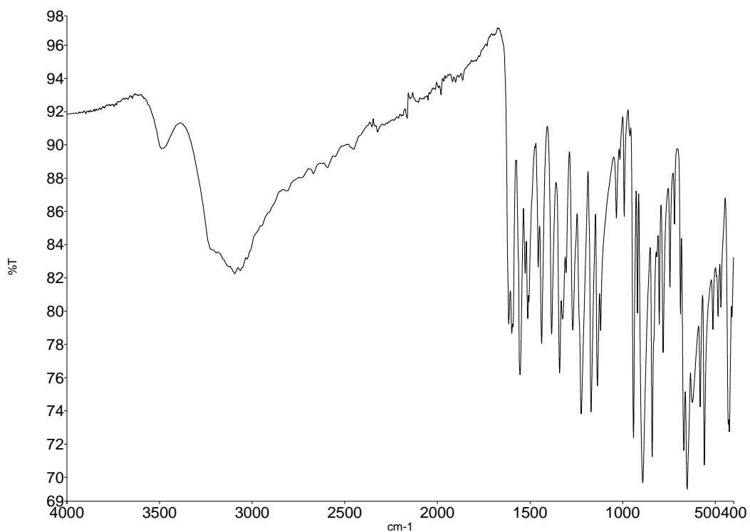
**Slika D21.** Infracrveni spektar kompleksa  $[\text{MoO}_2(\text{4OHSal-4HBOH})(\text{H}_2\text{O})]$  dobiven sintezom uz refluks u acetonu s  $\text{H}_2\text{4OHSal-4HBOH}$  ligandom
