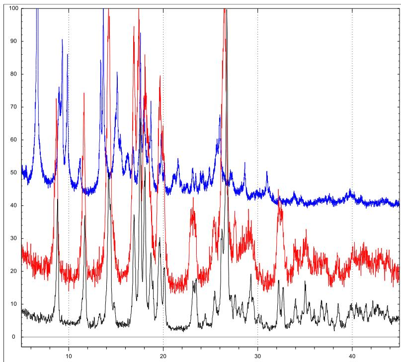
**Slika 24.** Difraktogrami prahova: spoj dobiven metodom A u acetonu s  $\text{H}_2\text{OHSal}$ - $4\text{HBOH}$  ligandom (crno),  $[\text{MoO}_2(\text{4OHSal-4HBOH})(\text{H}_2\text{O})]$  (crveno),  $[\text{MoO}_2(\text{3OHSal-4HBOH})(\text{H}_2\text{O})] \cdot (\text{CH}_3)_2\text{CO}$  (plavo)
