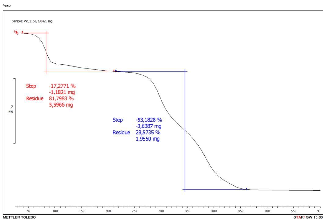
**Slika 30.** Termogram kompleksa  $[\text{MoO}_2(\text{3OHSal-4HBOH})(\text{H}_2\text{O})] \cdot (\text{CH}_3)_2\text{CO}$
