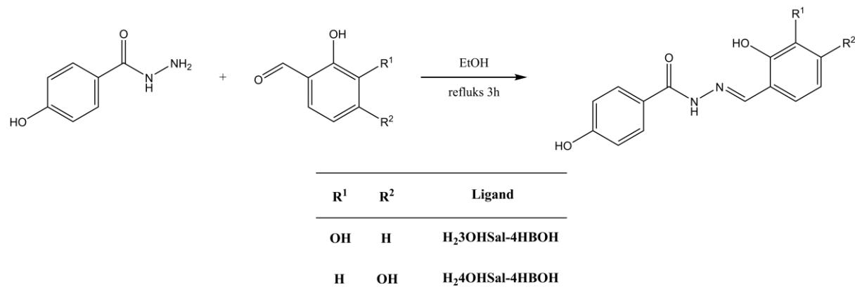
Shema 1. Sinteza hidrazonskih liganada  $H_2^3OH\text{Sal-4HBOH}$  i  $H_2^4OH\text{Sal-4HBOH}$
