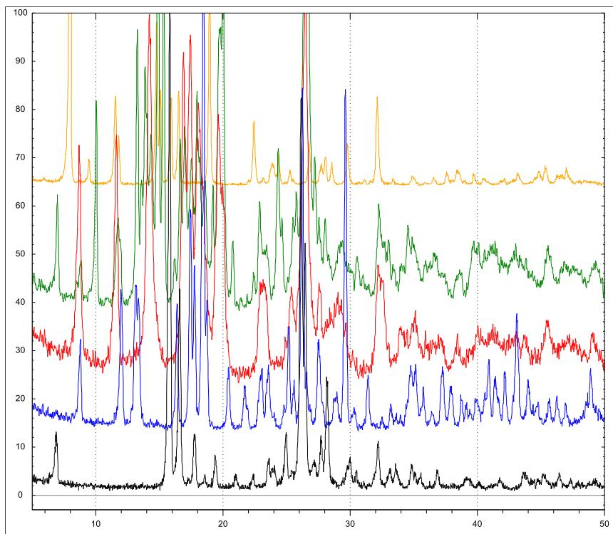
**Slika 27.** Usporedba difraktograma liganda i prahova kompleksa priređenih s  $\text{4OHSal-4HBOH}$  ligandom:  $\text{H}_2\text{OHSal-4HBOH}$  (crno),  $[\text{MoO}_2(\text{4OHSal-4HBOH})(\text{EtOH})]$  (plavo),  $[\text{MoO}_2(\text{4OHSal-4HBOH})(\text{H}_2\text{O})]$  (crveno),  $[\text{MoO}_2(\text{4OHSal-4HBOH})(\text{H}_2\text{O})] \cdot \text{MeOH}$  (zeleno),  $[\text{MoO}_2(\text{4OHSal-4HBOH})]_n$  (narancasto)
