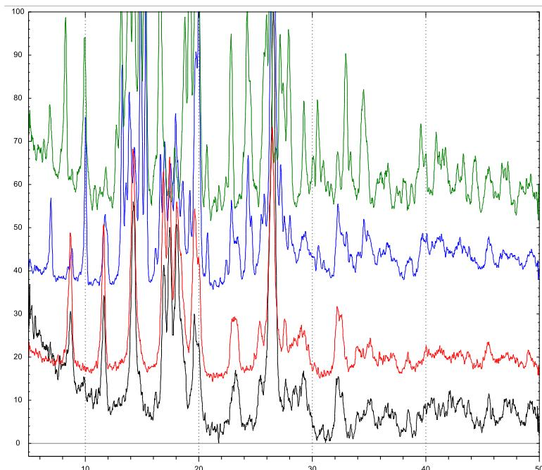
**Slika 21.** Usporedba difraktograma prahova kompleksa reakcijom s  $\text{H}_2\text{OHSal-4HBOH}$  ligandom u metanolu:  $[\text{MoO}_2(4\text{OHSal-4HBOH})(\text{H}_2\text{O})]$  (metoda A; crveno),  $[\text{MoO}_2(4\text{OHSal-4HBOH})(\text{H}_2\text{O})] \cdot \text{MeOH}$  (metoda B; plavo),  $[\text{MoO}_2(4\text{OHSal-4HBOH})(\text{H}_2\text{O})]$  (metoda C; crno) i metoda D (zeleno).
