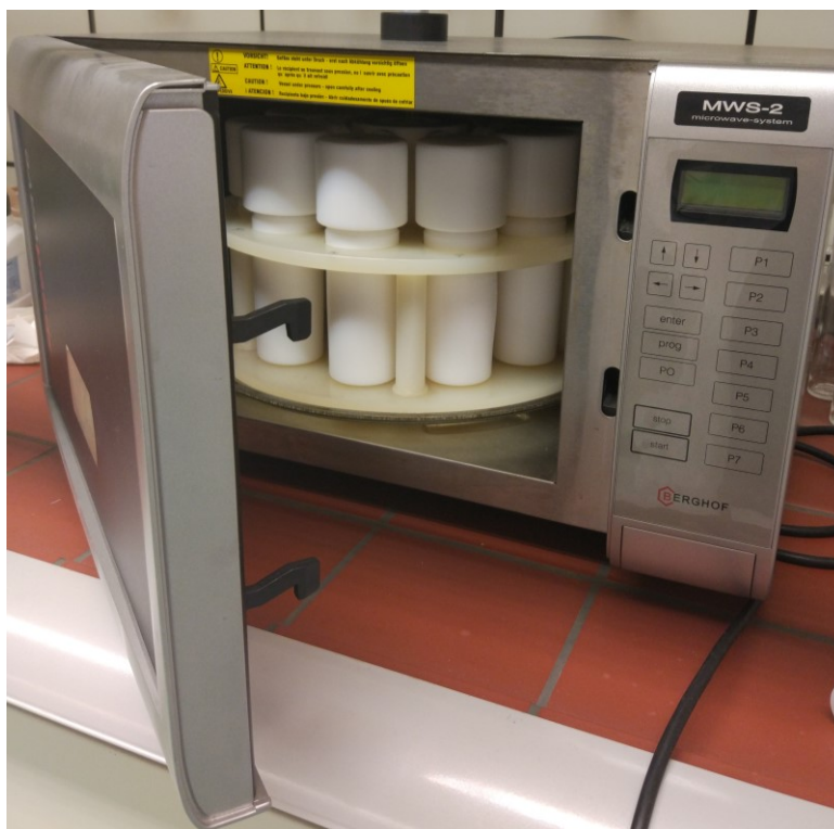
Slika 12. Uređaj MWS-2 Microwave System Speedweve Berghof
