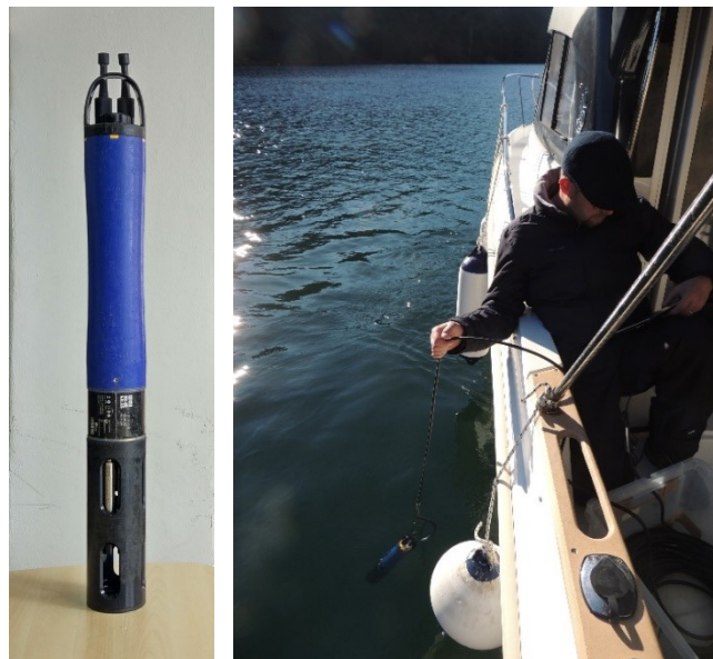
Figure 4.4. Multi-parameter probe EXO2 (YSI) (left), and the measurement of the water physico-chemical parameters by using the probe (right)
