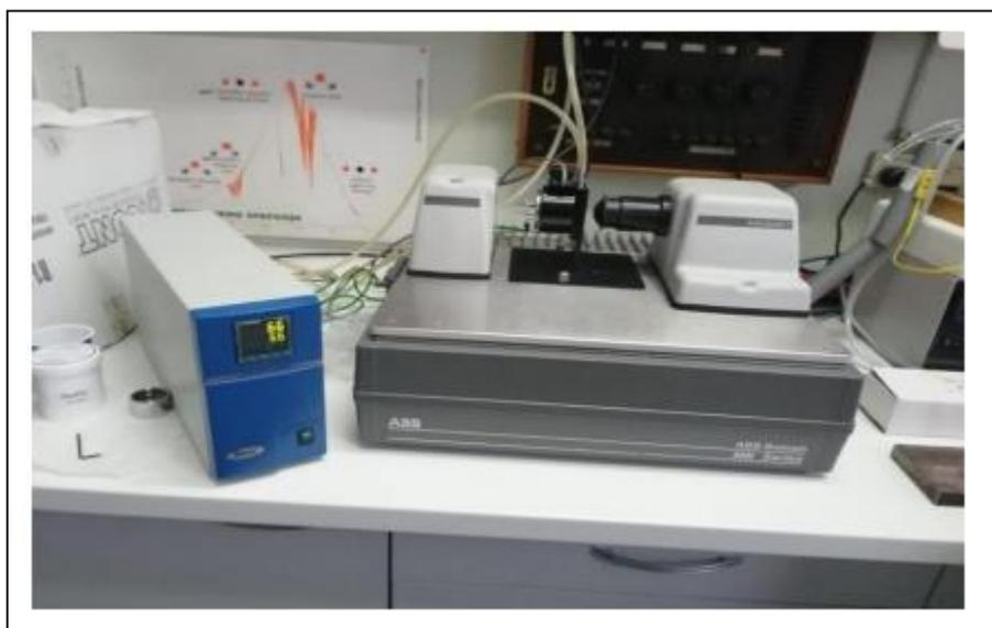
Slika 11. FT-IR spektrometar ABB Bomem MB102 i grijač s regulatorom temperatura Specac 3000 Series.<sup>20</sup>
