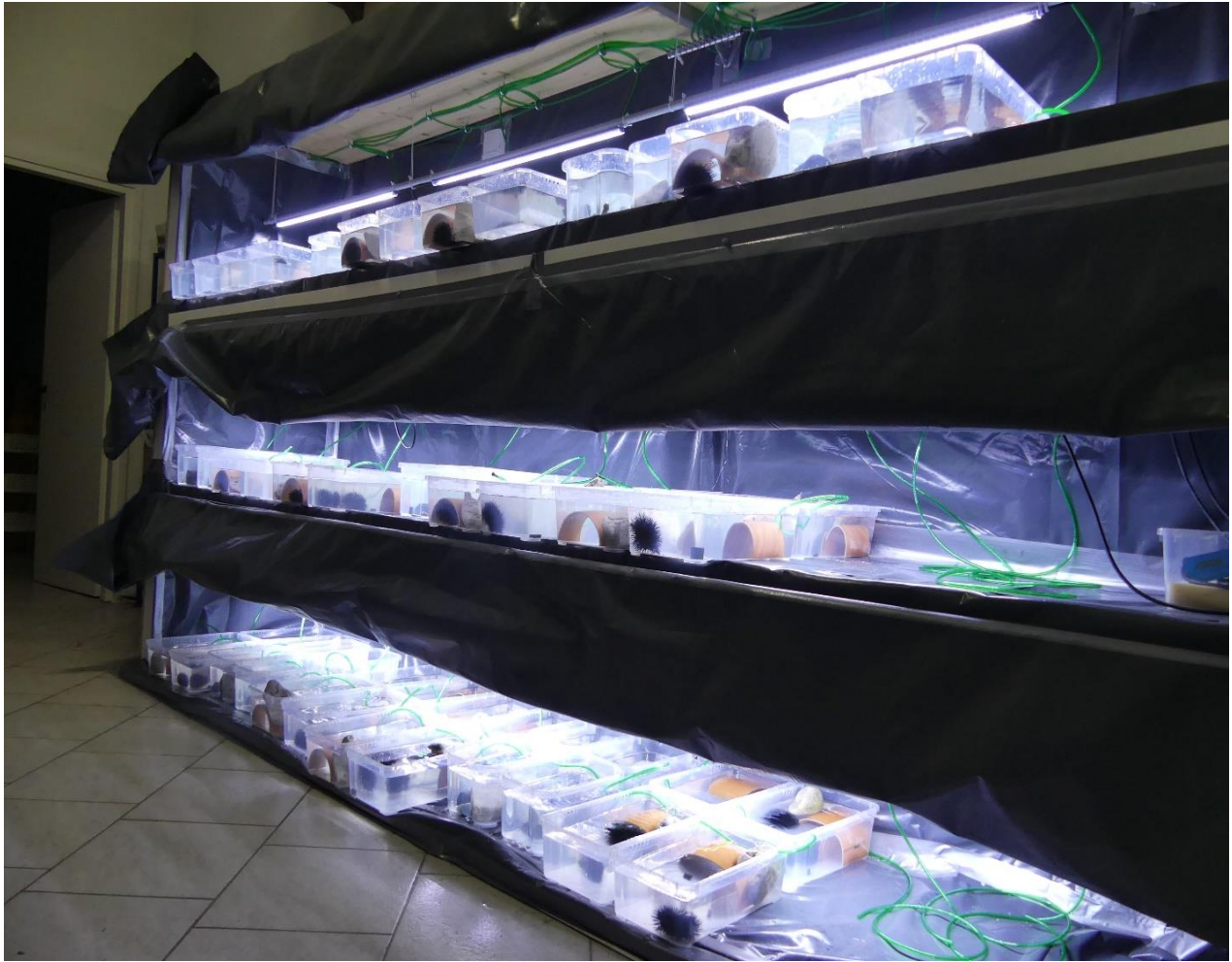
Figure 8. Shelf setup in which different light regimes are established on different shelf levels. The upper shelf contains the "None" treatment level, the middle shelf contains the "Full-night" treatment level, and the lower shelf contains the "Half-night" treatment level.
