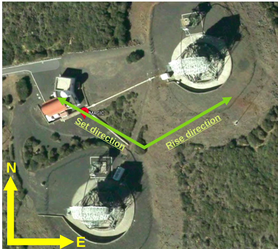
Figure 3.3: Photo showing the configuration in which the source can be observed. In this case the rise and set direction of the Crab Nebula are shown. Better stereo performance is obtained in the set direction as the telescope baseline is greater in such case as opposed to observing in the rise direction case.
