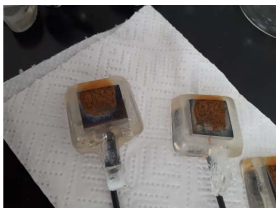
Figure 1. Appearance of carbon steel sample before testing
