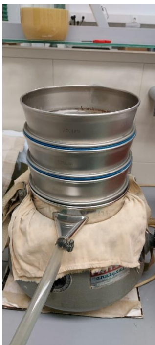
Slika 12. Tresilica marke Fritsch, modela Analysette
