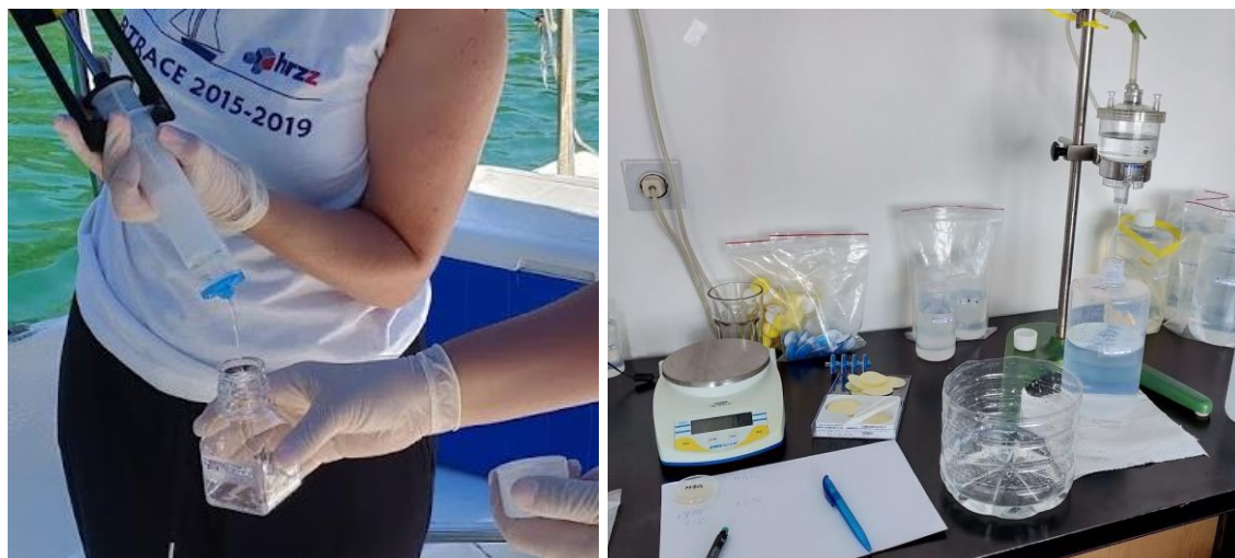
Figure 3.6. On board filtering (left) and polycarbonate filtration system for filtration under nitrogen pressure (right).
