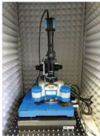
Figure 24. Photograph of AFM used at IFZg.
