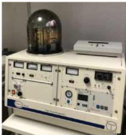
Figure 21. Metal evaporator at IFZg.
